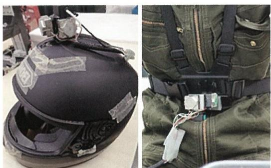
(a) Head and human three axis angular velocity meter
